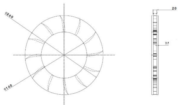
Fig.1. 2-D Model of Impeller
