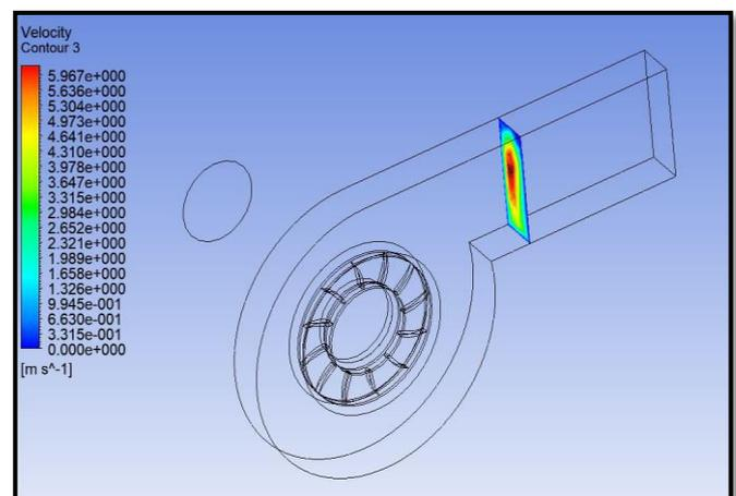
Fig.3(a). Outlet Velocity Plot
