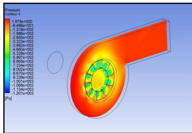
Fig.3(c). Overall Pressure Plot
